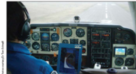
Dr. Tom Schell at the controls of an A-36 Bonanza during flight tests of the new Synthetic Flight Bag (SFB). The SFB provides a supplemental attitude instrument with digital terrain and other data.
